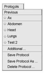
When a new image set is loaded, an initial protocol is selected according to the scan protocol name and body part DICOM tags of the loaded images. Use the Protocols menu to select another display mode from a list of MPR display protocols:
